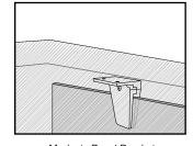
Modesty Panel Bracket Attaches underneath work surface with fasteners (included)
